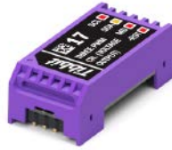
#17 Three PWMs with power outputs
