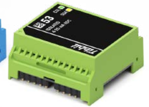
#53 Isolated four-channel 4-20mA ADC
