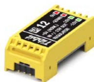
#12 +15V/-15V supply for Tibbits #13 & #14
